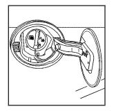
The tethered fuel cap is located behind a hinged fuel door on the passenger's side of the vehicle.
